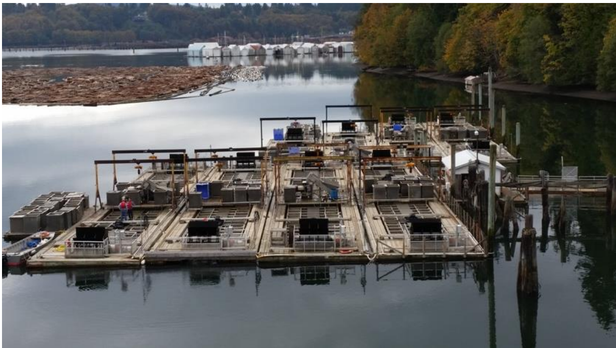
Fig 14. A large shore-based FLUPSY system located in WA State consisting separate rafts; each raft is powered by a paddlewheel that generates an upwelling current through the base of large bins holding shellfish seed (photo used with permission by Taylor Shellfish Company).
